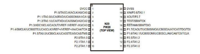
Pin 18 and Pin 19 are XIN and XOUT and allow an external crystal to be connected, either 32kHz or a fast crystal. Given the small number of pins, this is all that's available on this device.
