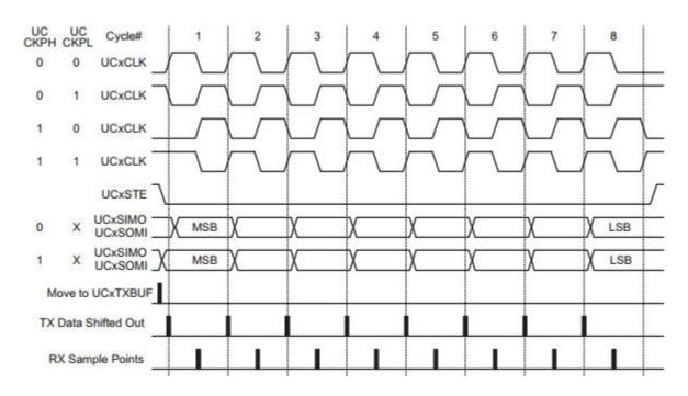
Its important that the right phase and polarity are selected so that the slave and master both capture the bit at the correct clock transition. If this configuration is not correct, you will see garbage coming out, and the slave will not properly receive the data sent by the MSP430. For example, we can see the SPI interface specifications for the CC1101 transceiver:
