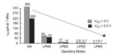
At 1MHz, we go from 300uA down to less than 1uA by switching to LPM3. This is what makes the MSP430 such a good microcontroller for low power applications. It can survive for years on batteries. But, to take advantage of this, we have to build an application that takes advantage of these low power modes and turns on only what's necessary when it's necessary.
