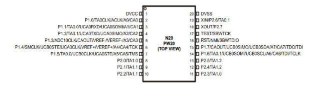
Looking at the pins in the diagram we notice that each pin has a long name, with several designations separated by a slash. Because microcontrollers have a limited number of pins and
