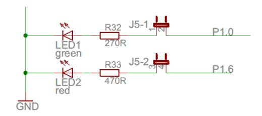
You can see the Launchpad board has two LEDs at P1.0 and P1.6. Each LED has a series resistor with a different value to make the output luminosity more uniform when they are lit.
