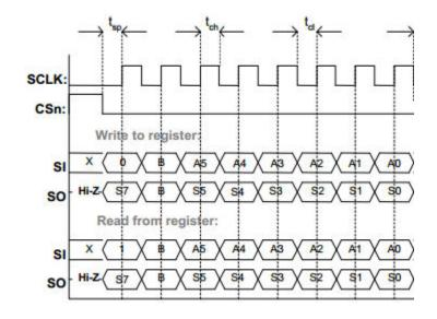
The CC1101 needs to sample with a rising edge clock at the center of the bit time. Clock Phase = 1 and Phase = 0 are the correct MSP430 master settings in this case.
