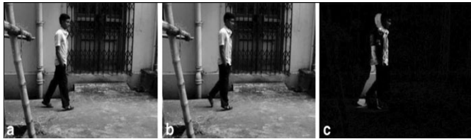
Fig.5. Temporal frame differencing. (a) Present Frame (PF) (b) Previous Frame (Prev) (c) Result = PF – Prev
